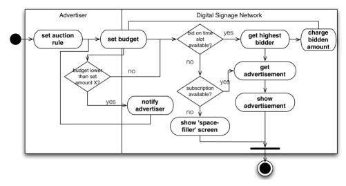
Figure 1. An exemplary rule set integration for digital signage (UML activity diagram)
